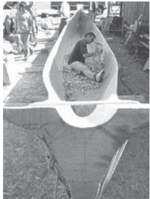
Calvin Hunt uses an elbow adze to hollow out the Comax nation's canoe. The sides will be steamed out to add a foot to the beam.
